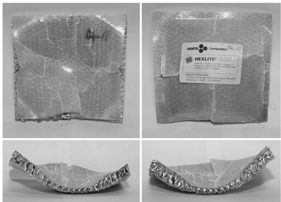
Fig. 13 Damage inflicted on Hexlite 620 for hemispherical impactor (clockwise from top left: top surface, bottom surface and cross sectional views)—Specimen 150 × 150 mm
